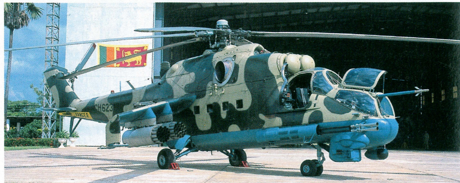
Below: This Mi-35P was one of the first two delivered in July 1998. It is seen here outside the hangar the unit was sharing with 7 Squadron at Hingurakgoda-Minneriya in early 1999. The big Sri Lanka flag emblazoned on the hangar is evidence of the personnel's fierce patriotism. Note the Mi-35P is armed with four rocket pods as well as the 12.7mm Gatling gun in the nose.
