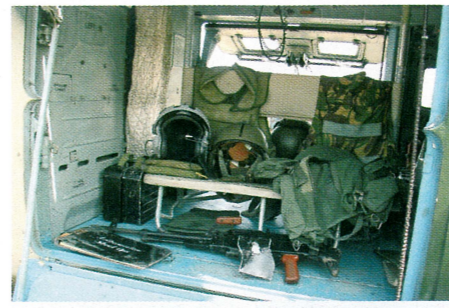
Above: The gunner's position – note the Kevlar protection on the seats.
