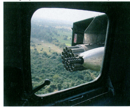
Below: A close up of the 80/57mm rocket pod and a 23mm gun pod that SLAF aircrew used during the war.
