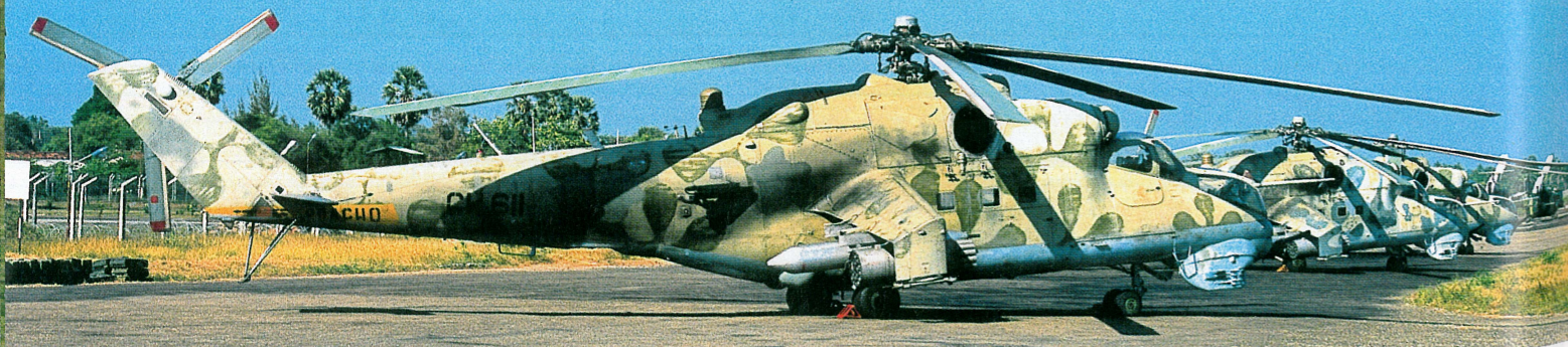
Below: All three leased Mi-24Vs sit on the ramp at Hingurakgoda-Minneriya in early 1996. Of the 26 Mi-24/35s that have been flown by the SLAF, there are two main variants; the Mi-24V and Mi-35P. The original three were the earlier Mi-24V with a 12.7mm Gatling gun mounted at the front, which were bolstered through the purchase of another four Vs before the Mi-24Ps (which the SLAF refer to as Mi-35Ps) and newer Mi-35Ps arrived, with the 30mm gun running alongside the starboard side of its fuselage. Due to the two types being used, the SLAF refer to the whole fleet as Mi-24/35s.
